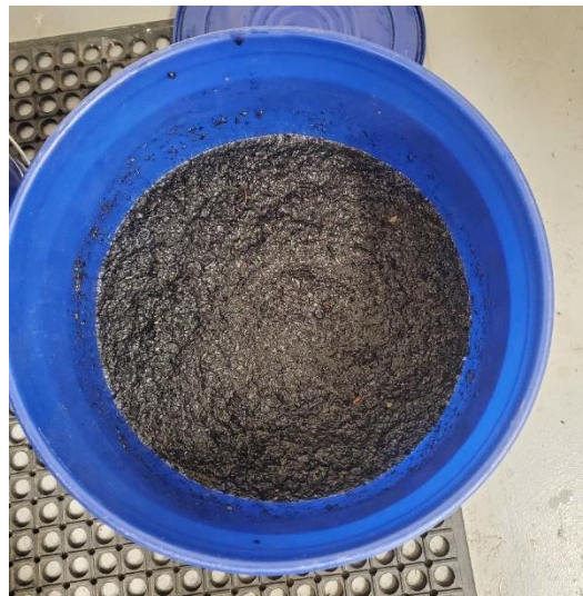
Biochar charging in anaerobic digester effluent
